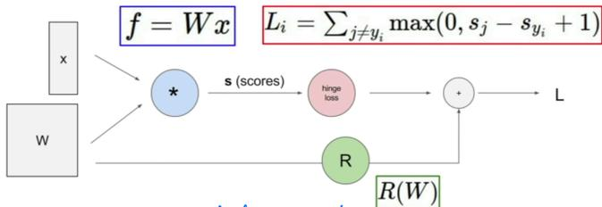
important to calculate gradient for neural network (complex function)
