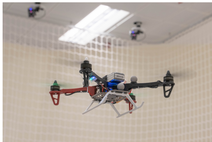
Figure 9. F330 quadrotor UAV used for flight experiments.
